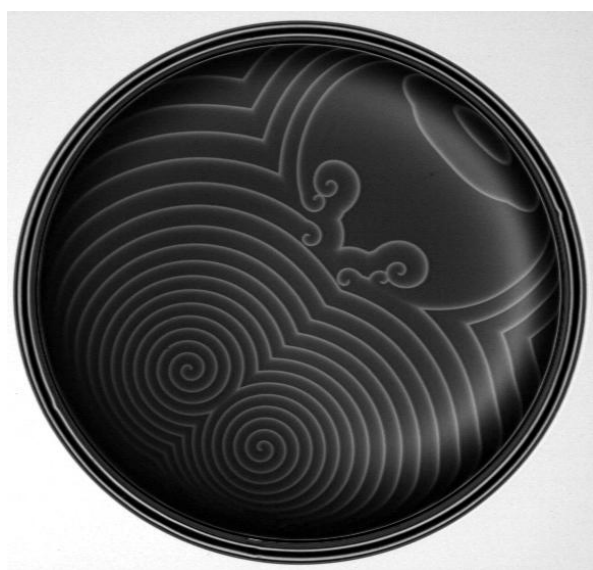
The non-linear, oscillating nature of the Belousov-Zhabotinsky Reaction can be observed in real time. Reproduced with permission from Niklas Manz.
